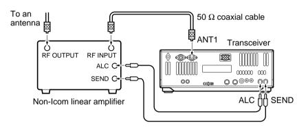
The specifications for the SEND relay are 16 V DC 2 A. If this level is exceeded, a large external relay must be used.
