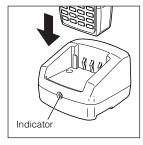
The red indicator turns off when the charge is completed. Remove the battery pack from the basket.
