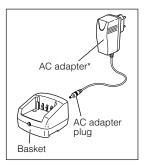
Mount the battery (with or without being attached to the unit) in the basket as shown. Turn off the unit while charging.
