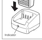
4. After charging time is elapsed (page 52), remove the battery pack from the basket. The red indicator stays turned on as long as the pack is mounted on the basket regardless of the charging status.
